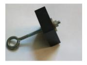
The second method I use for all my Science Olympiad bridges and towers. This method works for both top and bottom loaded bridges. First I take the leaf out of our old table, and simply lay the bridge over the gap. You can pull two tables close together if you don't have a table with a removable leaf. I then put a loading block on the bridge. The loading block I use comes from Pitsco, and follows the Science Olympiad
